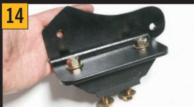
14 After making a template, we made the new engine mounts with some angle iron and a stock GM Turbo 350 transmission mount.
