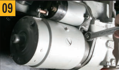
09 Installing the stock starter was a cinch, thanks to Bendtsen's research. Our stock flywheel had 166-teeth; they built this one to replace it.
