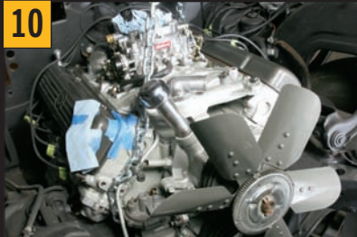
10 After a little creative trimming and hammering, we reinstalled the original 394ci V-8.
