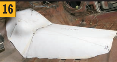
16 To assist in recreating our transmission tunnel, we worked with the folks at Tin Man Fabrication. The Tin Man made a three-piece paper template before building it out of sheet metal.
