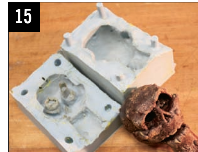
15 After the appropriate cure time, we separated the two halves and removed our wax skull. Upon close inspection, you can see that silicone picks up remarkable detail.
