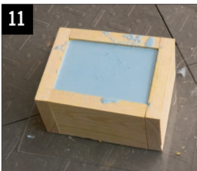
11 After letting our first side of the mold set for 16 hours to cure, we flipped our box over and removed our clay from the original.
