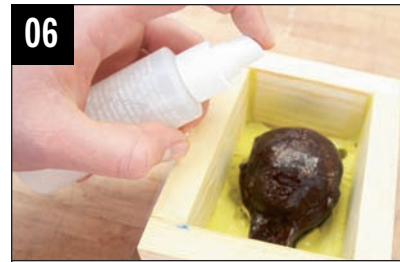
06 With urethane RTV molding material, using mold release is a must. A light misting with silicone RTV will ensure easy release.
