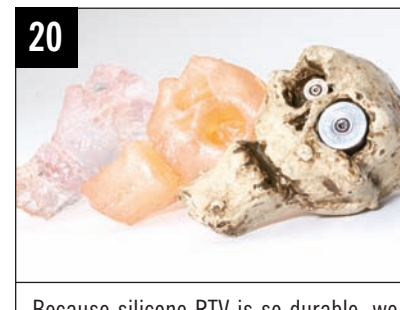
20 Because silicone RTV is so durable, we were able to do multiple pourings and get the same detail out of it. You can usually get about 20 castings out of a mold before the detail begins to diminish.
