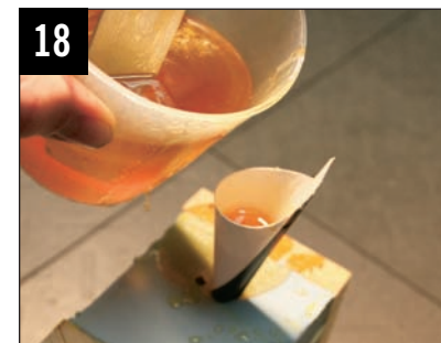
18 We poured our dyed resin into the pour spout slowly, allowing all the gases to escape out of the air vent. We continued pouring until resin came out of the vent.
