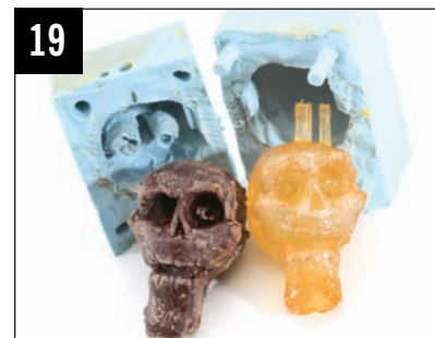
19 After the appropriate cure time (usually between two to ten hours depending on thickness), we had an exact replica of our original sculpted skull.
