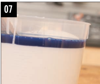
07 Silicone RTV is a two-part compound. The silicone itself (white) and a hardener (blue) are mixed in a 10:1 ratio.
