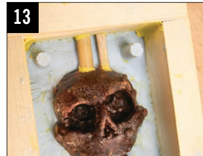
13 If an object is completely encapsulated by the silicone, you will need to add a pour spout and an air vent at the highest point of the object. We used wooden dowels.
