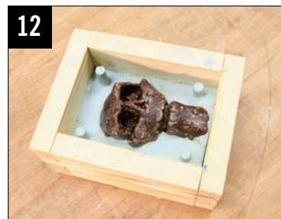
12 As you can see, the depressions in the clay formed the male end of the keyway and our original part is secured snugly in the first mold half.
