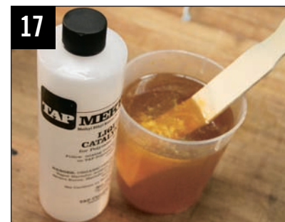
17 For our final casting, we used a polyurethane compound, which like our silicone RTV is a two-part resin. We used a clear resin, which allowed us to add dyes and pearl flakes.
