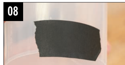
08 To reduce air bubbles in our molding material, we cut a small hole in our separate mixing cup and covered it with tape. This allows air pockets to pop in the mold pouring process. If air bubbles set next to our original object, they will cause imperfections in our final casting.
