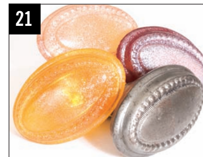
21 Here is another example of the casting process. We took an antique doorknob that would be at home in any traditional rod and casted it in multiple colors.
