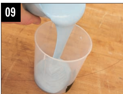
09 We used the two-cup mixing method. After mixing in one cup, we transferred it to another to move the material stuck to the sides of the first cup to the inside of the new cup.
